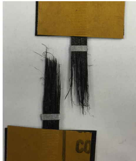
Figure 3-3: Fully failed CNT yarn composite specimen.
